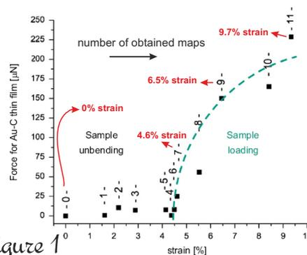
figure 1 Load versus strain curve after subtracting the PTP contribution. Strain percentage corresponding to fig 2 is shown
