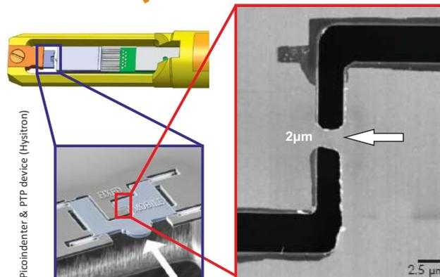
**The challenge:** *in situ* deformation of nanocrystalline metals to investigate the deformation mechanisms active during loading
