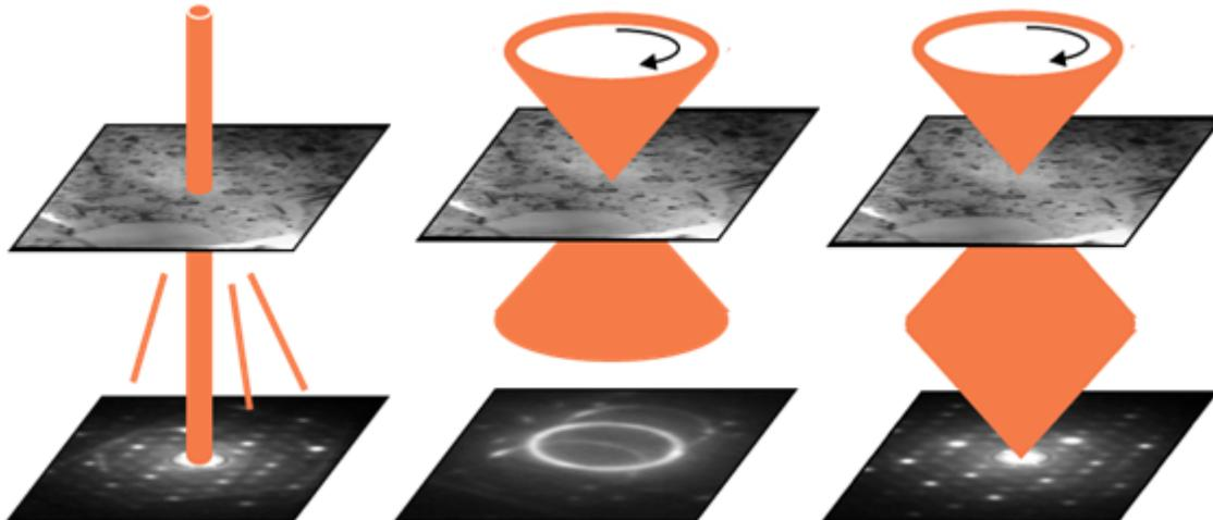
Fig. 2 (a) Conventional nanobeam illumination. (b) Precession illumination without complimentary descanning below specimen. (c) Precession combined with descanning below specimen.
