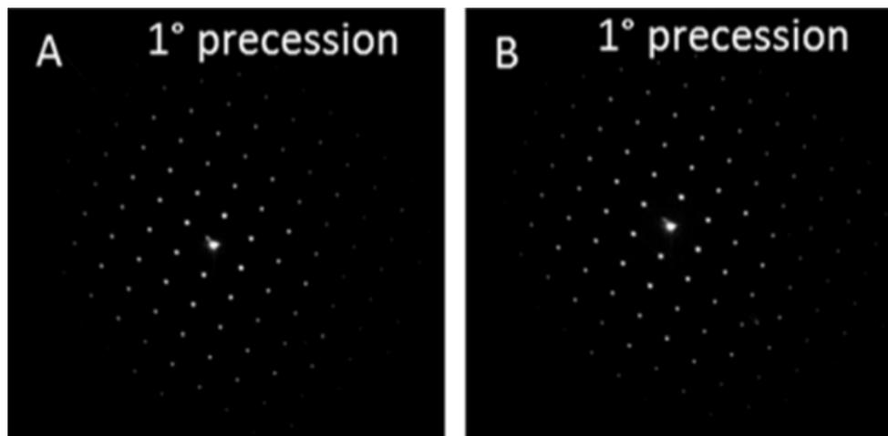
Fig. 3 Si <110> Diffraction patterns from the same region as shown in Fig. 1 with 1° precession.
