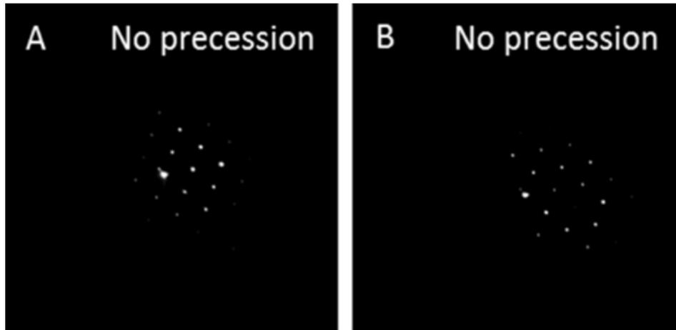
Fig. 1 Si  $\langle 110 \rangle$  Diffraction patterns from two nearby regions in a FIB sample. Note the strong intensity variations due to dynamical effects
