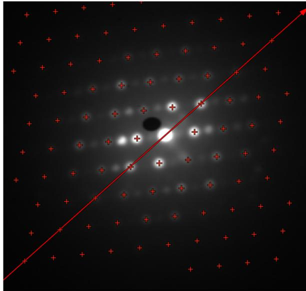
Fig. 4 Spot identification with Topspin strain analysis from a diffraction pattern with overlapping spots
