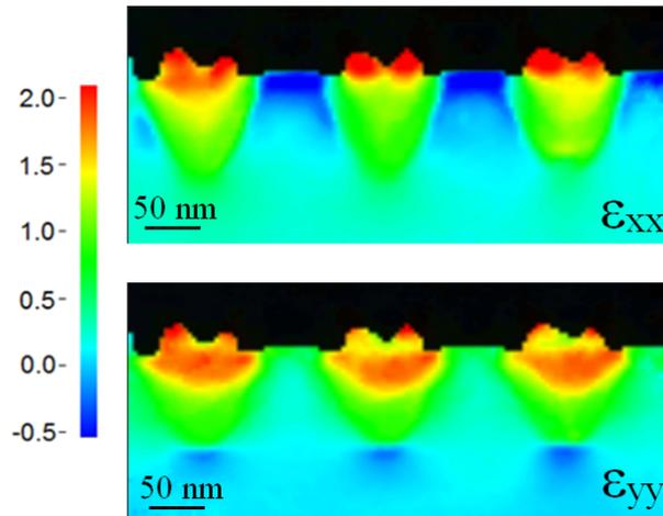
Fig. 6 Strain map from a p-FET device
