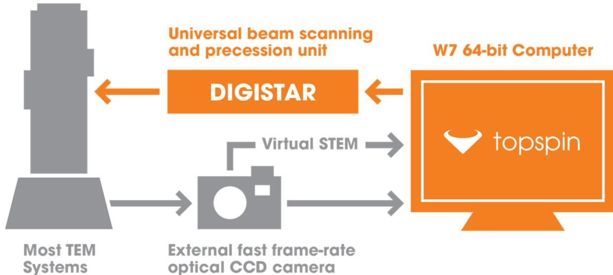
Fig. 5 Typical Topspin setup
